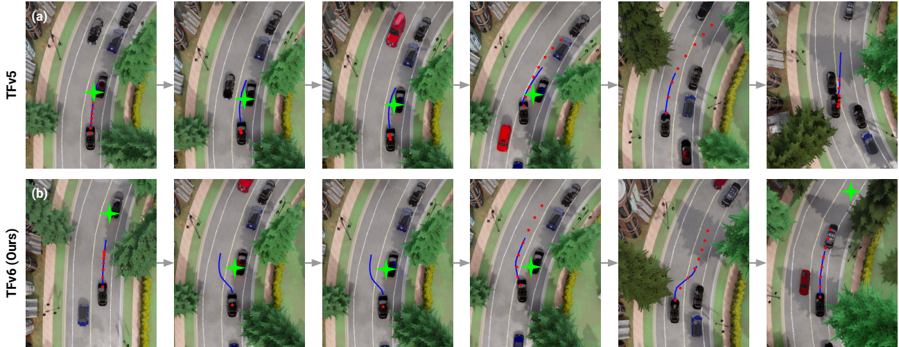
Figure 2. Target Point Bias. a) TFv5 outputs trajectories (red dots) and spatial paths (blue line) which are heavily influenced by the target point (green star). In situations such as overtaking static vehicles, this results in unrealistic and unsafe trajectories that pass dangerously close to the static vehicles. b) With the modifications incorporated in TFv6, we observe that the model is less prone to this bias.
